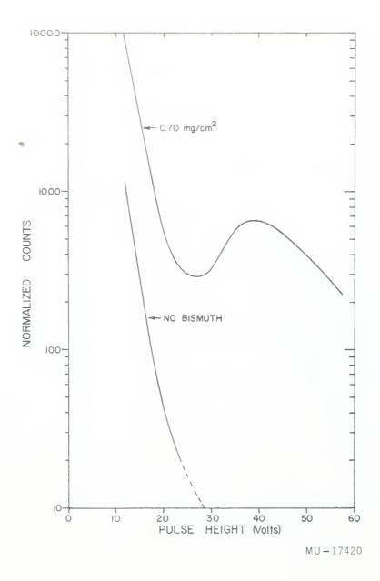
Fig. 10. Comparison of the differential pulse-height spectra for the no-bismuth and 0.70-mg/cm<sup>2</sup> chambers.
